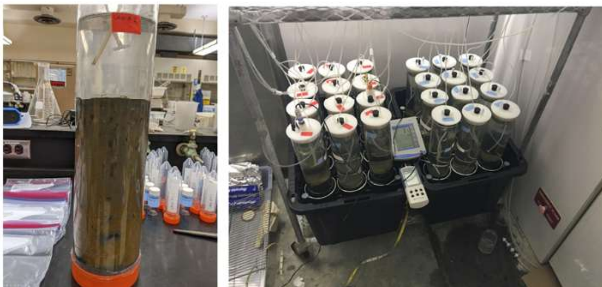
Figure 7.7.1. Sediment core and laboratory setup for the sediment incubation experiment
