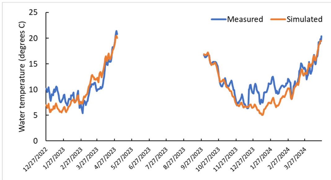
Figure 6.3.10. Comparison between daily observed (blue) and simulated (orange) water temperature for the Scotts Creek at State Route 29 gage.
