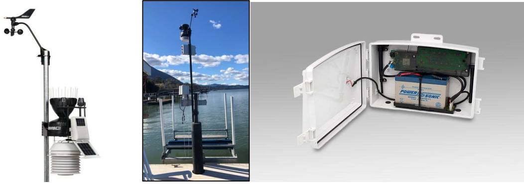
Figure 7.2.2. Weather station equipment (left-center) Davis Instruments Vantage Pro 2, and (right) Vantage Connect.
