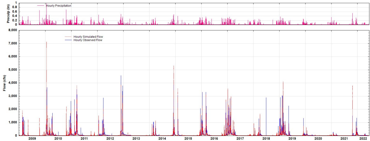
Figure 6.3.7. Hourly observed (blue) and simulated (red) streamflow, with precipitation in the auxiliary plot for the Scotts Creek at Eickhoff Road Bridge gage. cfs, cubic feet per second; in, inches.
